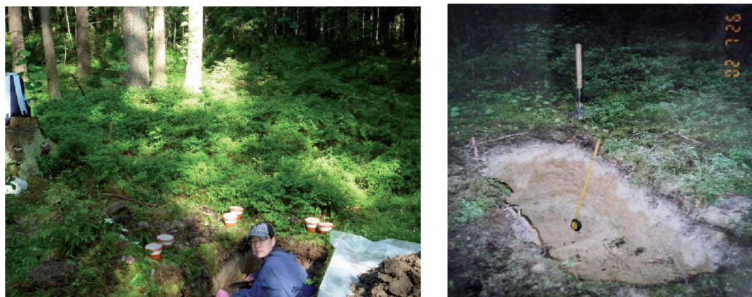
Fig. 4. Petrozavodsky permanent experimental plot in Karelia: a - SL installation by postgraduate student A. A. Petukhova: bilberry sphagnum forest plots (facies) (clearings - hollow depression) 14.07.2011; b - for comparison: the podzol profile in 2002, two years after the trees had been cut down: the beginning of the transformation of iron hydroxide hydrogels in the B 1 horizon (podzol evolves into marshy podzolic soil), 26.07.2002
