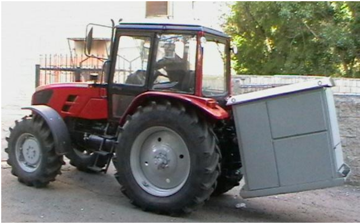
Figure 2. Electric generator driven by tractor (EGT) in transport position
