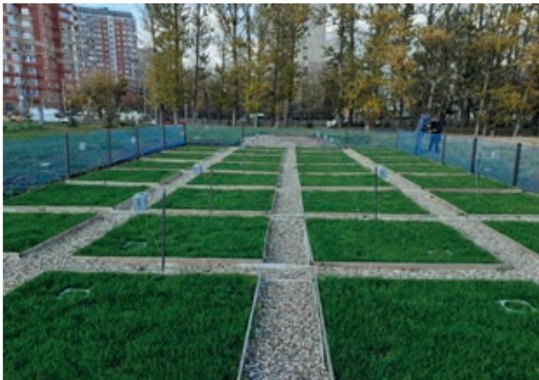
Fig. 3.2.2. The micro-plot field experiment with the bases of the over-ground exposure chambers.
