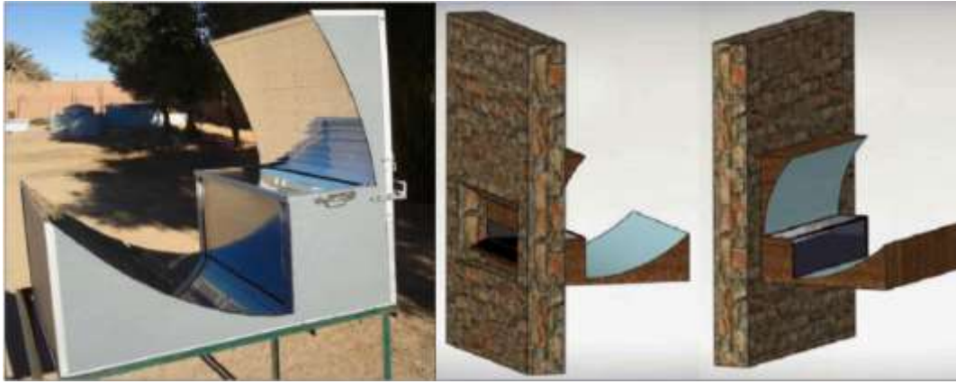
Fig. 3. Building integrated solar cooker [3]
