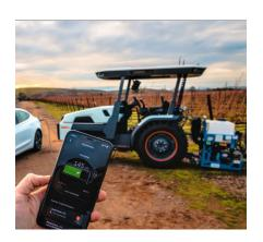
The tractor's 360-degree cameras help it avoid crashes, while its sensors allow it to collect and analyze over 240 gigabytes of data every day it works in the field. Farmers can receive updates from the tractor on their phone, including weather information from its built in weather station, as well as operation reports.
