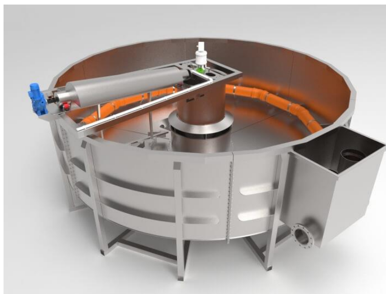
Fig 45 Radial flotation device: 1 – supply of condensate saturated with air; 2 – discharge of purified condensate; 3 – discharge of oil foam with water; 4 – discharge of sludge; 5 – switchgear; 6 – drive station – reducer for strokes; 7 – strokes; 8 – intake pipe for oil foam; 9 – steam supply for liquefaction and separation of oil from water in the intake pipe
