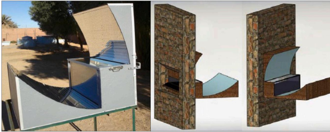
Fig. 3. Building integrated solar cooker [3]
